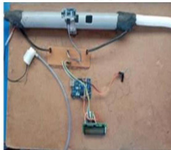
Fig: 6.3 Blocked and Overflow condition is displayed on LCD
