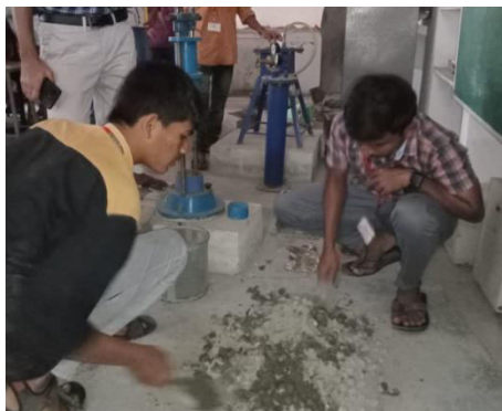
Fig. 2: Mixing of concrete.
