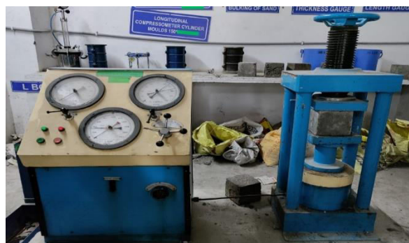
Fig. 6: Compressive strength test.
