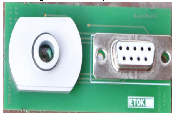
Figure 2: Fabricated cantilever with PVP material coating
