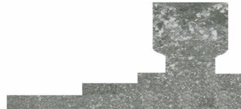
Figure 1. Gravity diecasting section having the process parameters: alloy-1, pouring temperature = 6750 C, mould pre-heat temperature = 2000 C, and degasified with 0.75%
