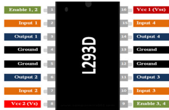
Figure 6. L293D Motor Driver
