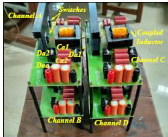
Fig. 5. Photograph of proposed 2kW interleaved converter
