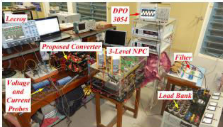
Fig. 11. Experimental set of proposed converter feeding energy to three phase three level NPC inverter
