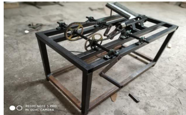
Fig 6.1. Assembled manual can crusher
