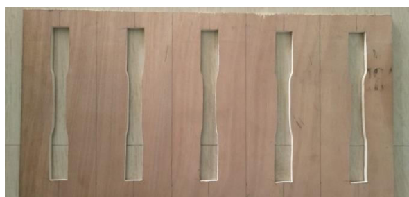
Figure 1 Dog-Bone shaped or dumbbell shaped specimen of 8mm thickness.
