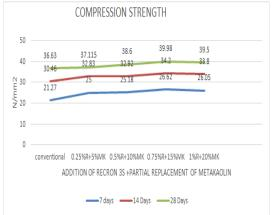
From the above experimental results, it is clear that the strength of concrete increases when the recron fiber is added and partial replacement of metakaolin with cement .It is found that the strength of concrete increases gradually from 0.25% to 0.75% and 5% to 15% of recron and metakaolin respectively At 1% and 20% of recron and metakaolin,
