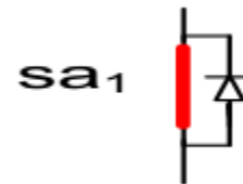
Fig.6. Shows the fault occurred due to the IGBT in Short condition.
