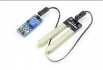
Fig 2: Soil Moisture Sensor ii) Light Sensor (LDR):
