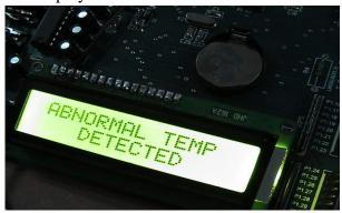
FIG 10 The displayed result when the patient exceeds the standard temperature value:
