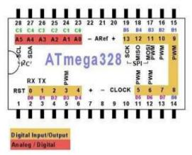
Fig:1: Pinout of ATmega 328
