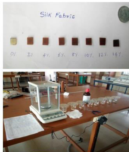
Figure 2. Glutaraldehyde with silk fabric in natural rubber specimens for benzene solubility test
