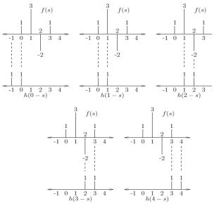
Fig2: Linear convolution by the graphical method.
