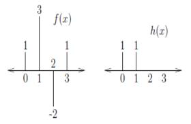
This convolution can be performed graphically by rejecting and shifting h(x), as shown in Figure 1. The samples of f(s) and h(s - x) that line up vertical are multiplied and summed:
