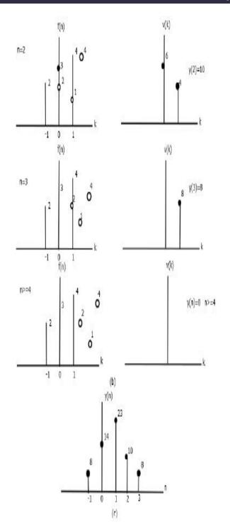
**Fig.3.1:** The sequences f(n) and g(n), shown in (a), are graphically convolved
