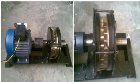
Figure 1: Induction motor with fluid coupling
