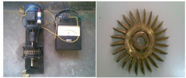
Figure 3: Wattmeter connected to motor
