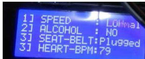
Figure4: If Alcohol isn't detected while driving then the speed is kept normal, Heart rate monitoring.
