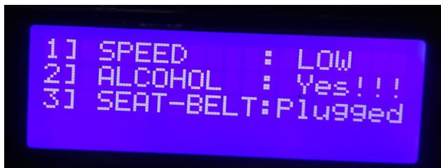
Figure3: Alcohol level detected while driving and automatically car speed slows down
