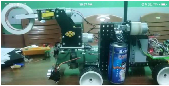
Fig 8. Pick and place arm in action.
