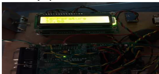
Fig 5: Temperature detection output display on LCD screen.
