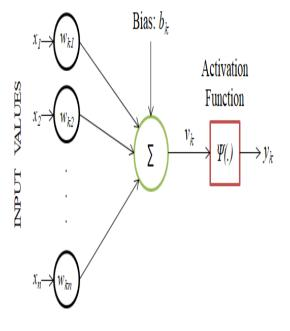
Fig. 1. Basic Architecture of Perceptron
