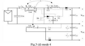
Once diode Do turns on, the series voltages of input source, capacitor  $C_2$ , leakage inductor, magnetizing inductor and secondary side supply output capacitor  $C_{Ol}$ . Also, by conduction of  $D_4$ , the output
