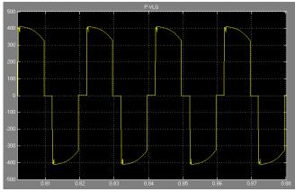
Fig. 9 Primary voltage waveform across the transformer
