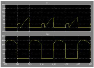
Fig. 6 Current and voltage waveforms in S1
