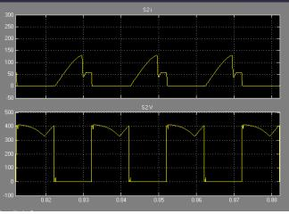
Fig. 8 Current and voltage waveforms in S2
