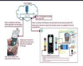
In hardware we are using Node MCU, Relay, Ultrasonic Sensor, Magnetic Float Switch Sensor and 12v motor.
