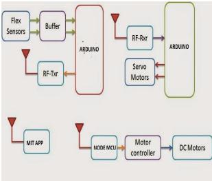
Fig 6: Flow Chart for Robotic vehicle The Fig 6 shows the working of the robotic vehicle and it can be done through the MIT app inventor. As per the code which was given to the node mcu microcontroller, it drives the motor driver to perform DC motors in a desired way in which we can control the robotic vehicle through our own instructions.
