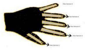
Fig 3: Flex Sensors Following fig shows experimental setup which consists of transmitter i.e. glove
