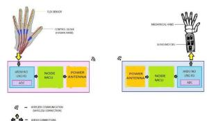
Fig 5: Flow Chart for Robotic Hand Here as in the Fig 5 shows the overall model of the robotic hand. The main mechanism
