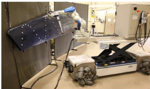
Mobile robot working on aircraft wing, courtesy Southwest Research Institute.
