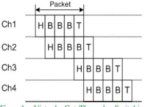
Fig. 4. Virtual Cut-Through Switching Technique
