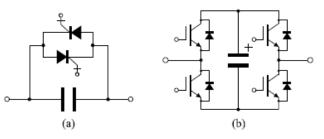
Fig. 1.1 Circuit configurations of two types of series compensators (a) GCSC (b) Voltagesource-type full-bridge compensator including SSSC and MERS
