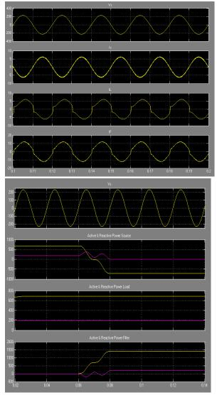
simulation results of the proposed converter under linear load conditions
