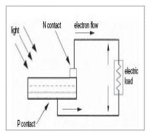
Fig 2.1: PV effect converts the photon energy into voltage across the pn junction
