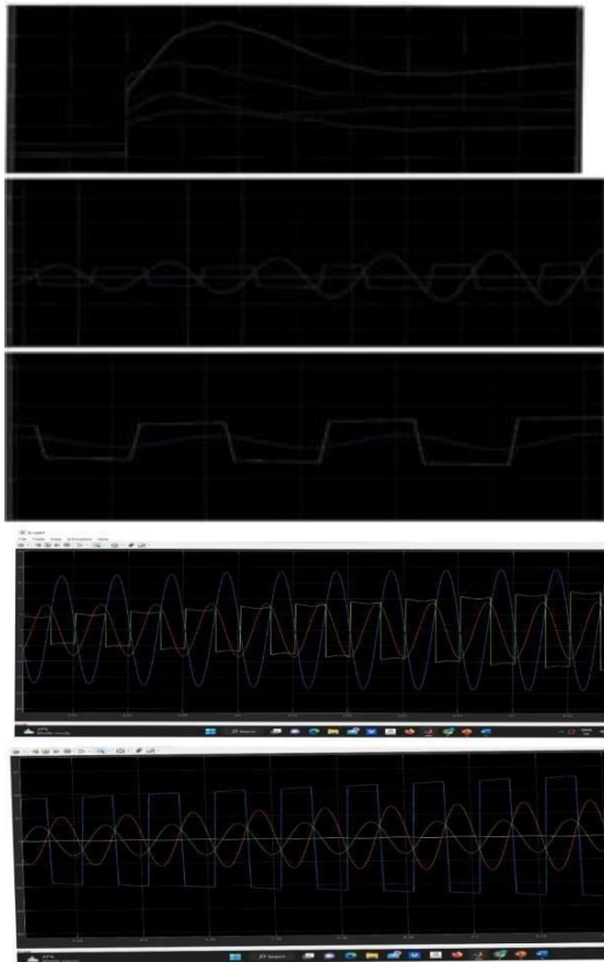
Fig3.4:LCC AC fault stimulation results
