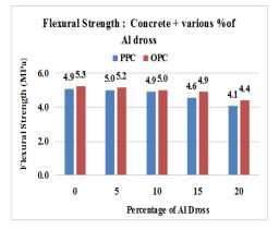
Figure 4. 19 28Days Flexural Strength Comparison for PPC And OPC mixes
