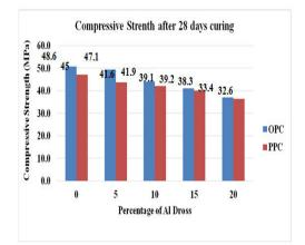
Figure 4. 13 variation of the compressive strength after 28 days of curing for OPC and PPC concrete at various percentage of Al dross
