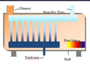
Figure 1: water tube boiler
