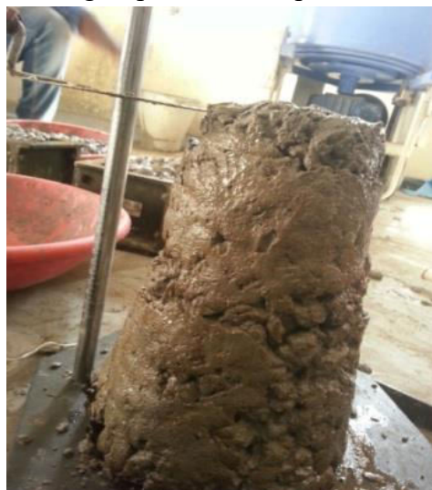
Fig. 4: Slump test on concrete.
