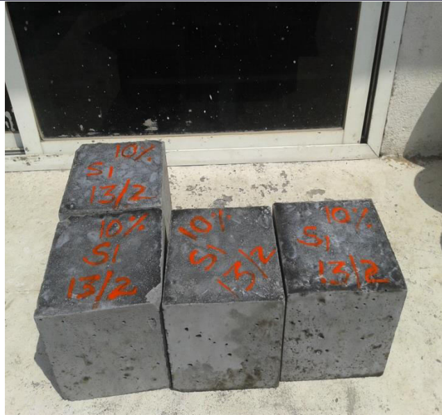
Fig. 3: SCBA Concrete cubes before drying.
