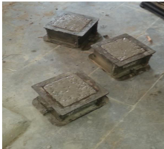
Fig. 2: SCBA concrete placed in cube moulds.
