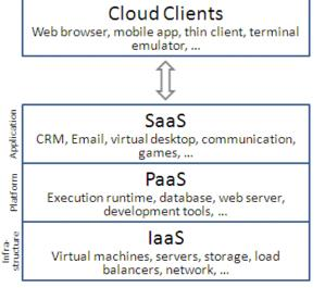
Fig 1: Cloud-computing layers accessible within a stack
