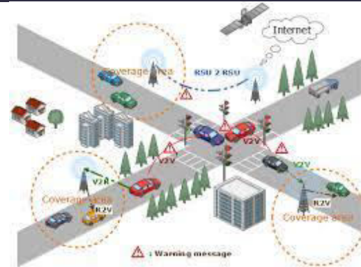
Figure.4.: RSU VANET Communication Model
