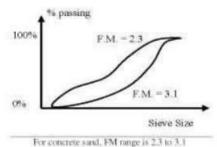
Fig.5. Graph showing fineness modules range for Concrete
