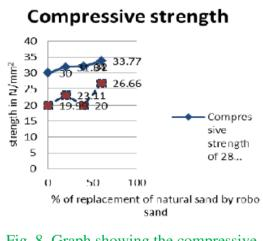
Fig. 8. Graph showing the compressive strength of concrete cured for 7 days and 28 days
