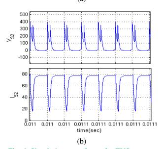
Fig. 6. Simulation waveforms for ZVS turn-on of the switches S1 and S2 at Vd = 80 V and Po = 400 W. (a) vS1 and iS1. (b) vS2 and iS2.
