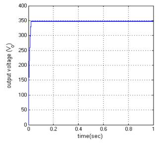
Fig.12.Output Voltage of Closed loop APWM full bridge Converter.
