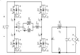
Fig.2.Circuit diagram of the proposed APWM full-bridge converter.
