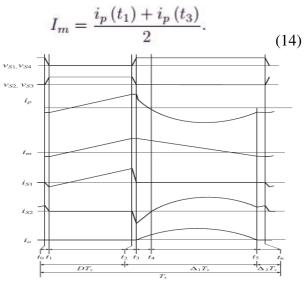
Fig.4.Theoretical waveforms of the proposed converter.
