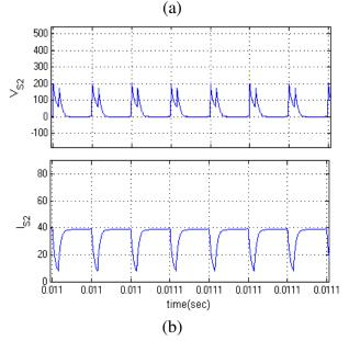
Fig. 8. Simulation waveforms for ZVS turn-on of the switches S1 and S2 at Vd = 40 V and Po = 400 W. (a) vS1 and iS1. (b) vS2 and iS2.
