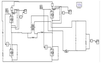
Fig.5.Matlab/Simulation model of proposed APWM Full Bridge Converter.
