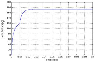
Fig.9.Simulation results for proposed converter output Voltage.
