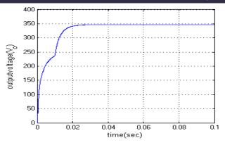
Fig.7.Simulation results for proposed converter output Voltage.
