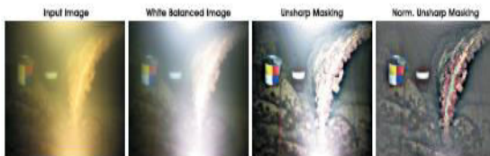
Fig. 7. Comparison between traditional unsharp masking and normalized unsharp masking applied on the white balanced image.
