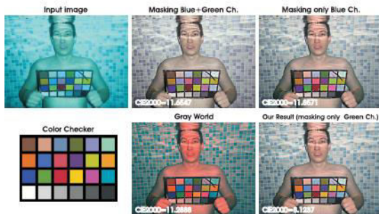
Fig. 3. Compensating the red channel in Equation (4). Since for underwater scenes the blue channel contains most of the details, using this information will reduce the ability to recover certain colors such as yellow and orange and also it tends to transform the blue areas to violet shades. Compensating the red channel by masking only the green channel (Equation (4)) these limitations are reduced significantly. This is confirmed visually but also by computing the CIE2000 measure using as a reference the color checker (displayed with white ink on the resulted images).
