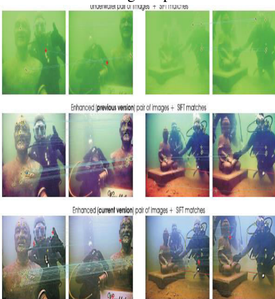
Fig. 16. Local feature points matching. To prove the usefulness of our approach for an image matching task we investigate how the well-known SIFT operator [72] behaves on a pair of original and dehazed underwater images. Applying standard SIFT on our enhanced versions (bottom) improves considerably the point matching process compared to processing the initial image (top), and even compared with our initial conference version of our proposed fusion-based dehazing method [35] (middle). For the left-side pair, the SIFT operator defines 3 good matches and one mismatch when applied on the original image. In contrast, it extracts 43 valid matches (without any mismatch) when applied to our previous conference version [35], and 90 valid matches (with 2 mismatches) when applied on the pair of images derived from this journal paper. For the right-side pair, SIFT finds 4 valid matches between the original images, to be compared with 14 valid matches for images enhanced with our initial approach [35], and 34 valid matches for the images derived from this paper.
