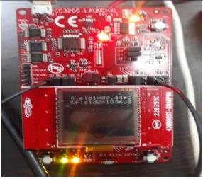
Figure 7: Temperature and Bed Occupancy data
