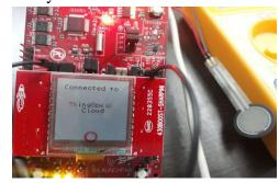
Figure 6: Hardware implementation of proposed system (CC3200, LCD Booster Pack, Pressure sensor).
