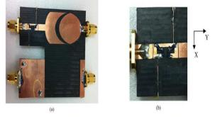
Fig. 3. (a) The fabricated prototype top layer (b) the integration of the PIN diodes switches.
