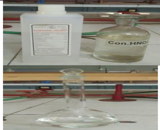
Ethanol and Con.HNO3 Conical Flask with 2% Nital
