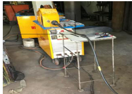
MIG welding machine Work pieces (MILD STEEL)
