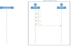
Figure 1 a watchdog timer that does not receive a heartbeat. It counts until reaching its
