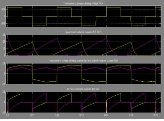
Simulation waveforms when V1 = V2 = 150 V, L1 = 200  $\mu$ H, L2 = 100  $\mu$ H.
