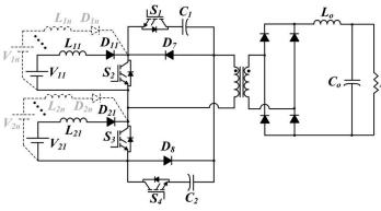
Fig. 1. Proposed multiinput isolated three-level dc/dc converter MULTIINPUT ISOLATED THREE-LEVEL DC/DC CONVERTER
