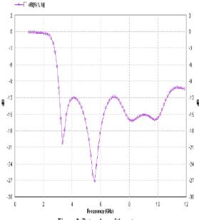
Figure 2: Return loss of the antenna
