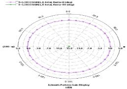
Figure 7: H-Plane Radiation pattern of the proposed antenna at 5.58 GHz
