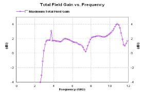
Figure 9: Proposed antenna Total Field Gain vs. Frequency
