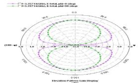
Figure 4: E-Plane Radiation pattern of the proposed antenna at 3.36 GHz.
