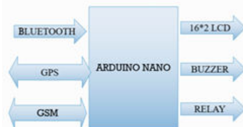
Fig 1.1: Block diagram of the proposed system
