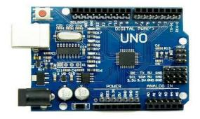
The Arduino Uno is the main processing unit of the system. It receives the distance data from the ultrasonic sensors and processes it to detect any cracks or defects on the track. The Arduino Uno is also responsible for controlling the motor that moves the sensors along the track.
