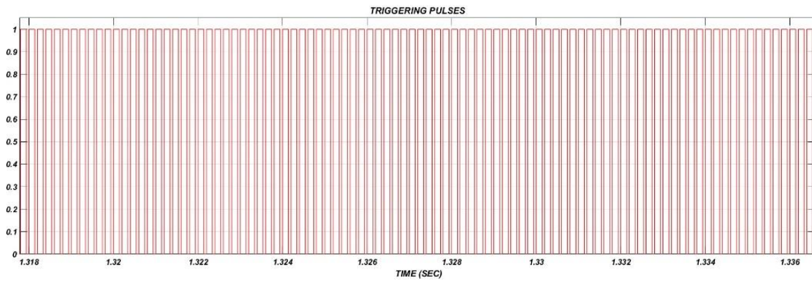
Fig.18 Triggering pulses to the Buck Boost converter
