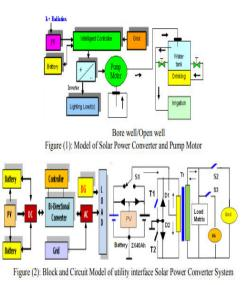
The converter works in bidirectional mode and performs both under charging and inverter mode of operation. The push pull configured centre tapped converter unit is switched ON and OFF alternatively in push pull mode by transistorized switching Power devices to produce ac power from the DC source.
