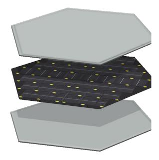
Figure 3. Layers of Solar roadway
