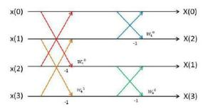
Figure 1. Signal Flow Graph of 4-point FFT 2. Error Tolerant Techniques for Parallel FFTs
