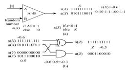
Fig.1. Stochastic logic, (a) Sequence generator scheme, (b) Stochastic signed multiplier.
