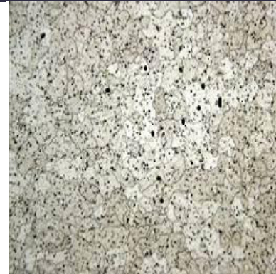
Fig-4: Microscopic view of the SSSC AA6061 inside the material with 100 magnification ratio.
