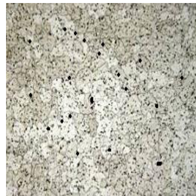
Fig-5: Microscopic view of the SSSC AA6061 inside the material with 100 magnification ratio.
