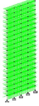
Fig: 5 Response spectrum loading along single grid
