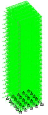
Fig:4 Response spectrum loading in 3D frame
